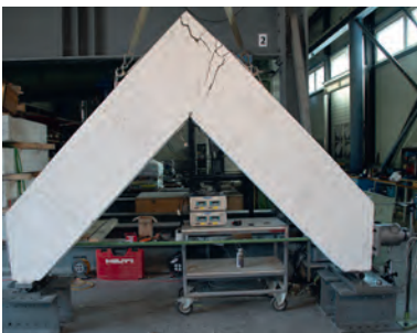
Fracture pattern of the test of a closing frame corner.
