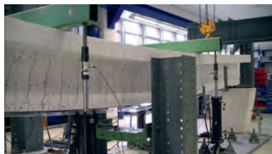
Four-point bend test of the untensioned beam strengthened with CRFP tensoning system.
