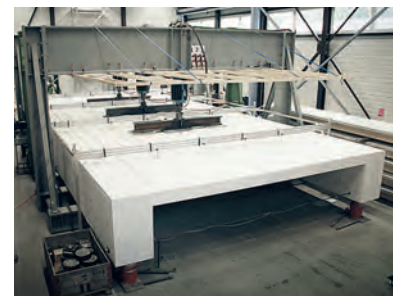
Fatigue test of bridge deck.
