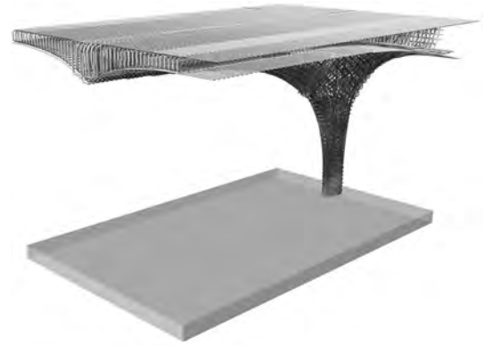
Fig. 4 Dreidimensionales Bewehrungsmodell. Three-dimensional reinforcement model.
