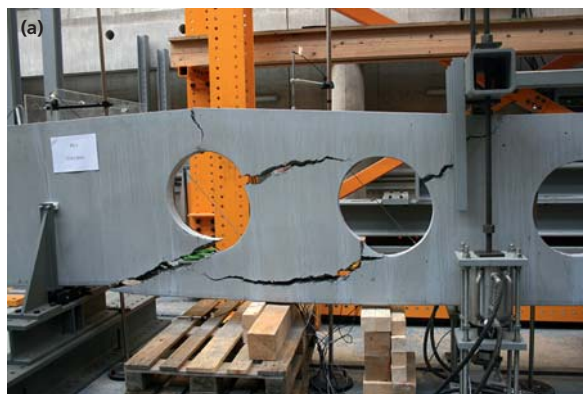
Fig. 8 Rupture des poutres PU3 (a) et PU5 (b). Cracking pattern at failure of PU3 (a) and PU5 (b).
