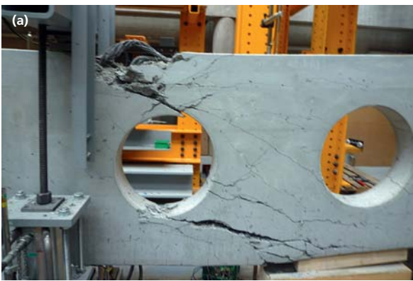
Fig. 13 Rupture des poutres PH6 (a) et PH7 (b). Cracking pattern at failure of PH6 (a) and PH7 (b).
