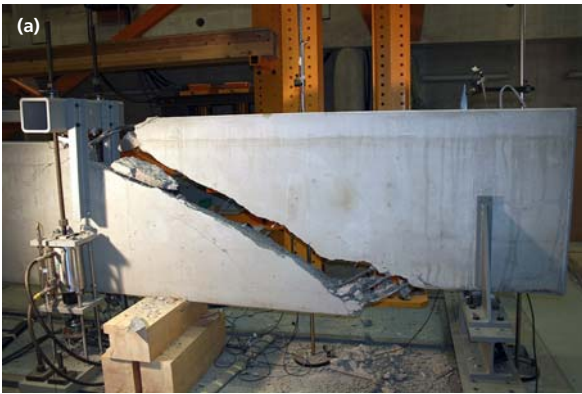
Fig. 12 Rupture des poutres PH1 (a) et PH4 (b). Cracking pattern at failure of PH1 (a) and PH4 (b).
