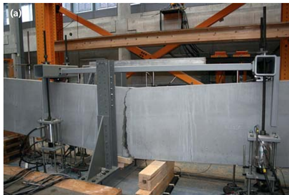
Fig. 7 Rupture des poutres PU1 (a) et PU2 (b). Cracking pattern at failure of PU1 (a) and PU2 (b).
